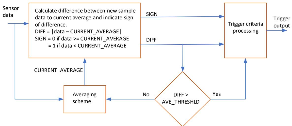
Figure 2. Sensor data algorithm to emulate a differential pressure sensor.
