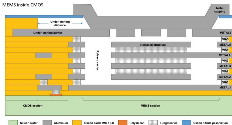
The cross sectional structure of NEMS: the MEMS within the CMOS technology
